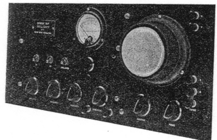
Fig. 3. A laboratory rule yesterday, a radiophone utility tomorrow. A modern simplified cathode ray oscilloscope.
