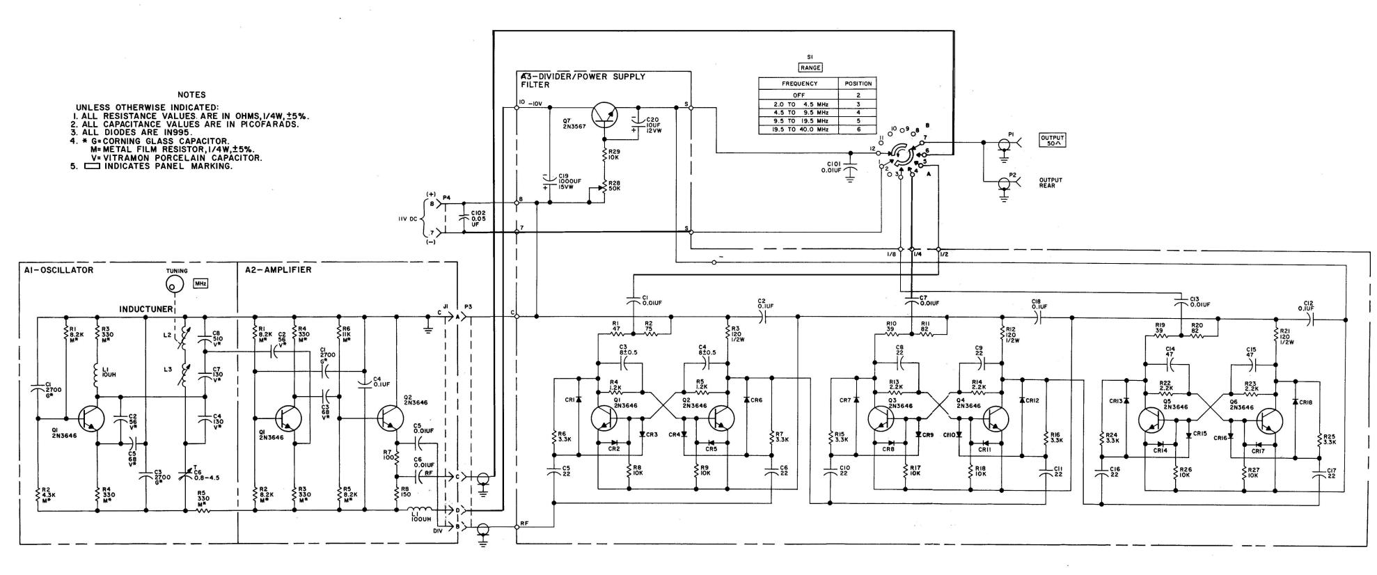
Figure 5-1. Tuning Head, Schematic Diagram
