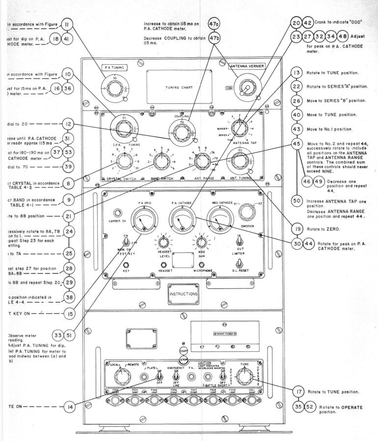
Figure 4-4. Tuning the Transmitter
