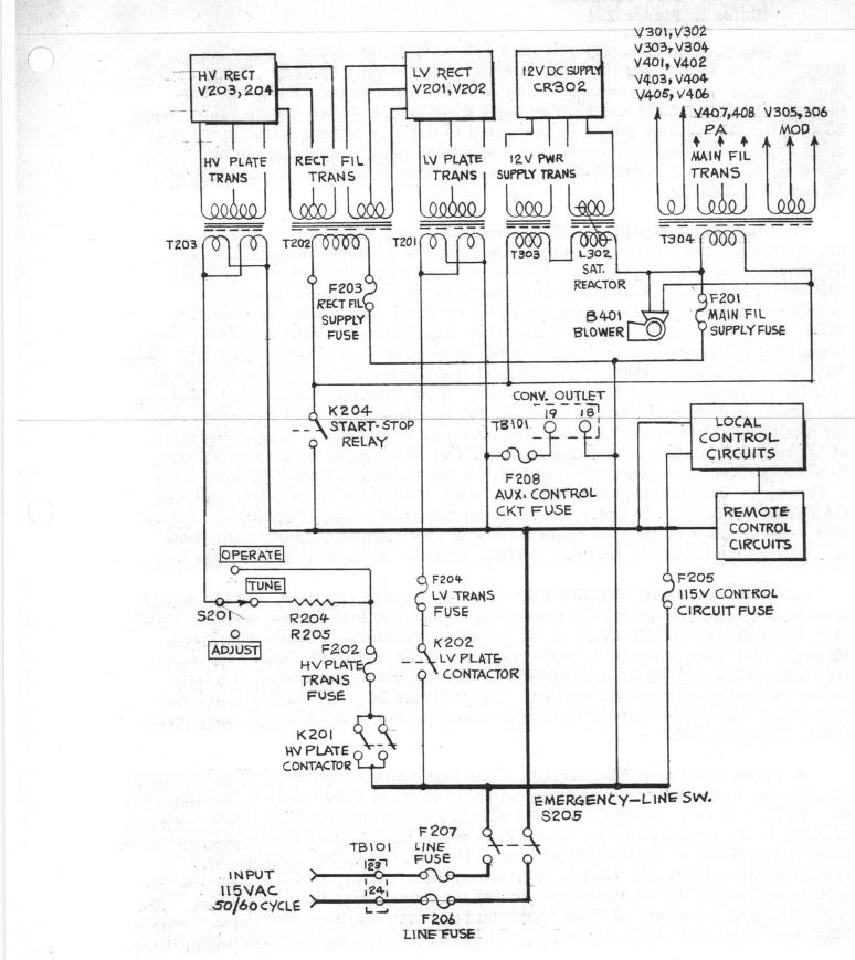
Figure 2-4. Power Distribution Circuit
