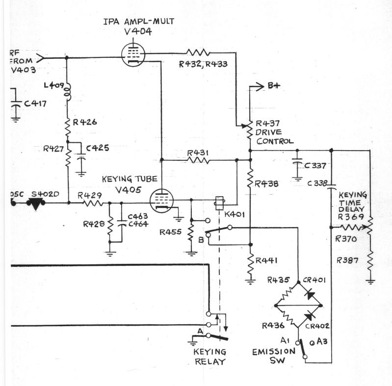
Figure 2-3. Keying Circuit
