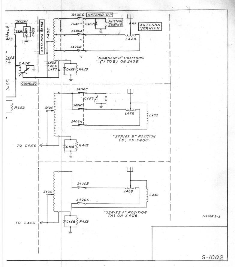
Figure 2-2. Simplified Radio and Audio Frequency Circuits
