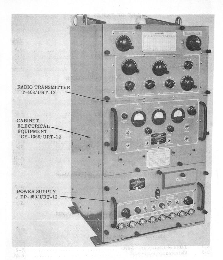
Figure 1-1. Radio Transmitting Set AN/URT-12, Relationship of Units
