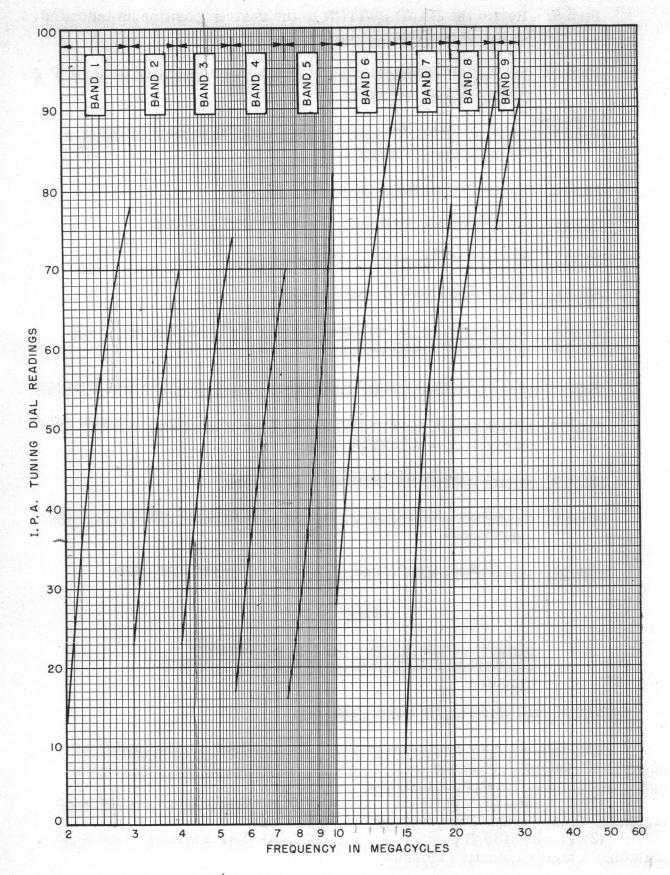
Figure 4-1. IPA Tuning Calibration (Typical)
