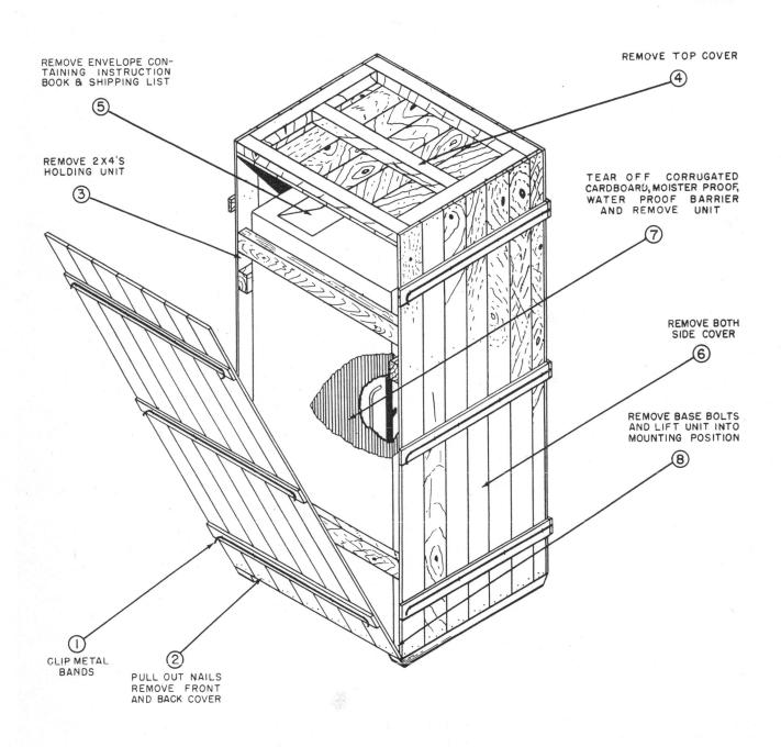
Figure 3-1. Unpacking Procedure
