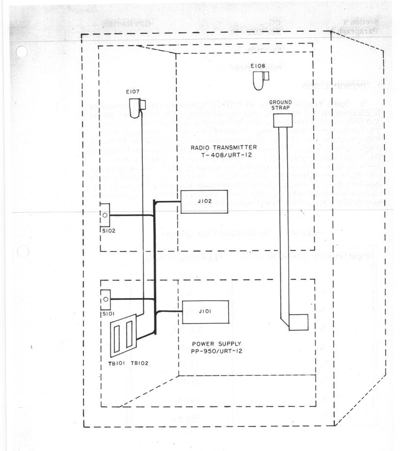
Figure 3-5. AN/URT-12, Internal Cabling Diagram
