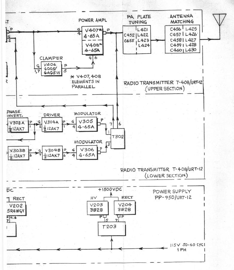
Figure 2-1. Radio Transmitting Set AN/URT - 12, Block Diagram
