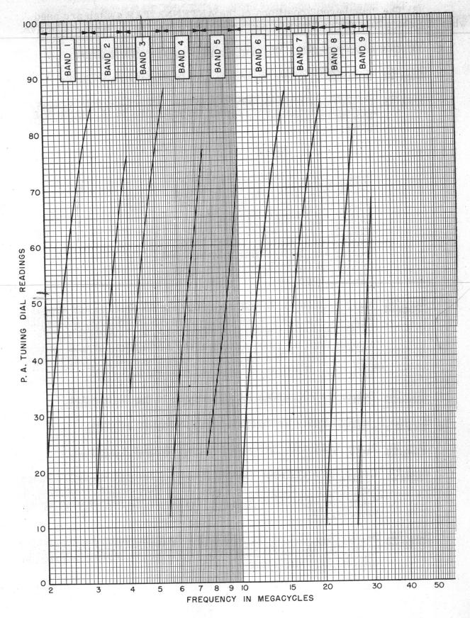
Figure 4-2. PA Tuning Calibration (Typical)
