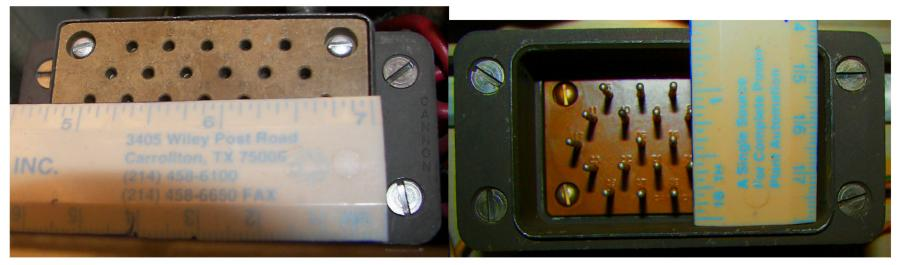
These images are of the connectors that mate the slide-out drawers to the frame cabinet. A jumper should be made for servicing the unit, with one of these on each end, so that the slide-out unit can be powered when extended from the cabinet.
