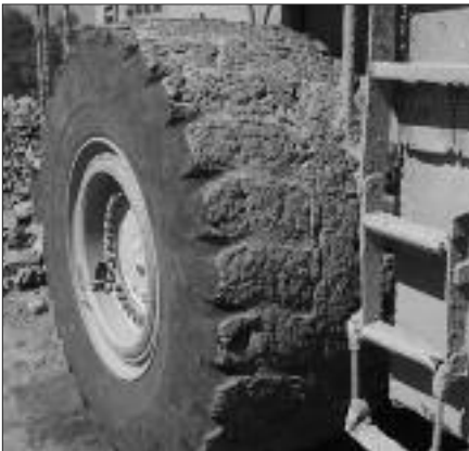
Fig. 10. This tire was worn smooth in 500 hours by spinning on abrasive material.
