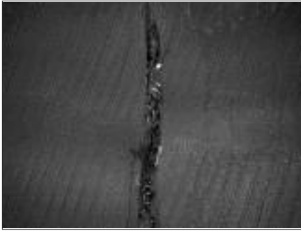
Fig. 14. This break resulted from a severe blow while overinflated.
