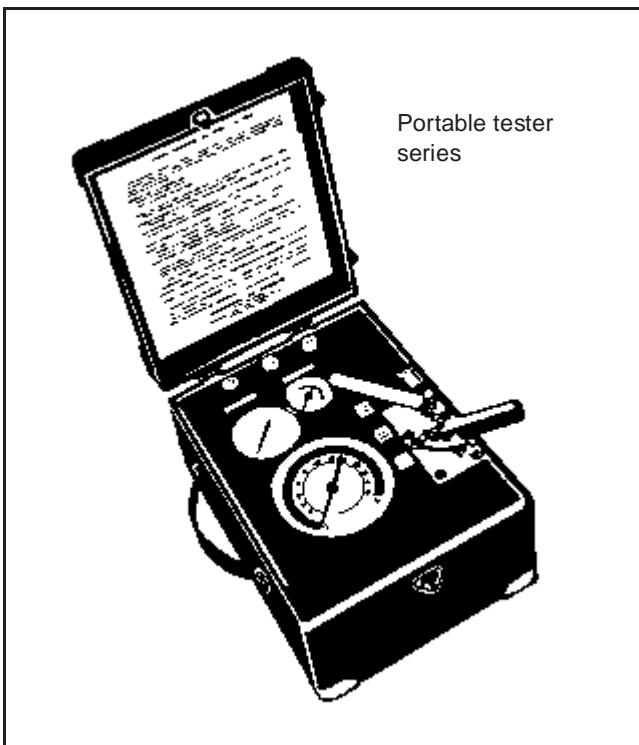
Figure 2-20. Portable hydraulic-circuit tester
