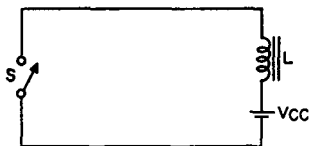
Fig. 85—Simplest form of deflection circuit.
