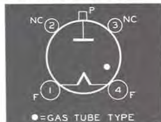
Bottom View of 816, 866A/866 Socket Connections
