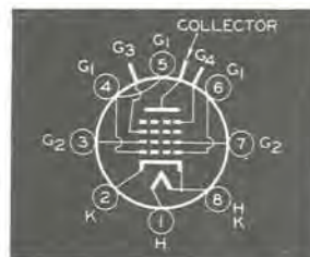
Bottom View of 825 Socket Connections
