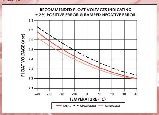
At temperatures greater than 40°C it is recommended that the same float voltage should be applied as that at 40°C with zero negative error permitted.
