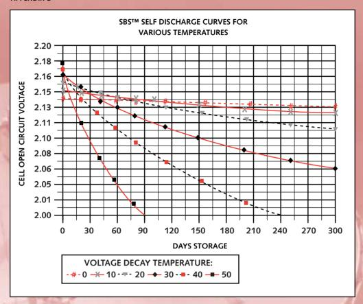
Based on a single 12V monobloc with 6 cells
